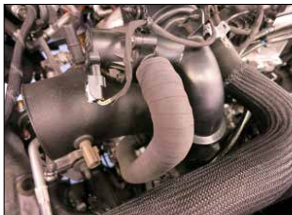
24. Install the BOV hose onto the BOV fitting. Do not secure with the spring clamp currently.
