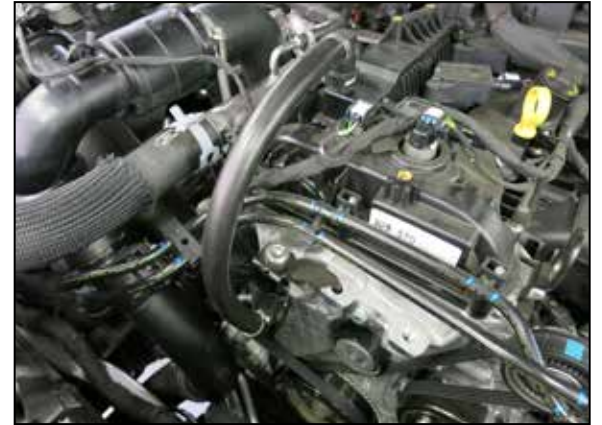
27. Install the CCV assembly onto the quick connect fitting installed into the K&N intake tube and on the valve cover as shown.
