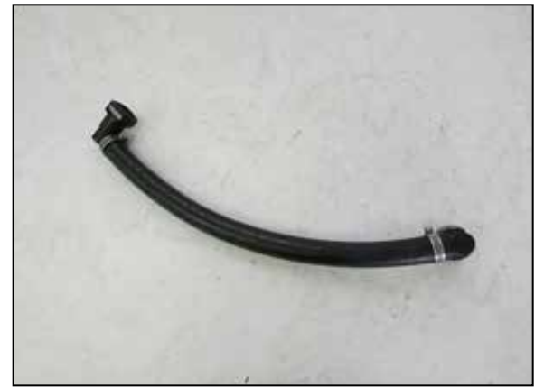
26. Assemble the CCV hose with the provided quick connect fittings as shown.
